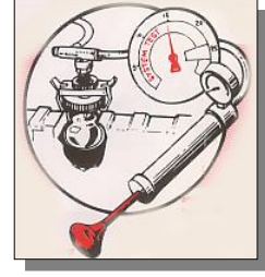
Pressuring the Cooling System
